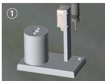
1 The probe moves to the sensor of the stylus cleaner.
