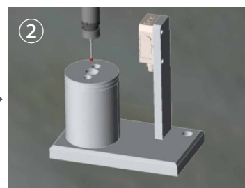
2 The probe moves to above the cleaner.
